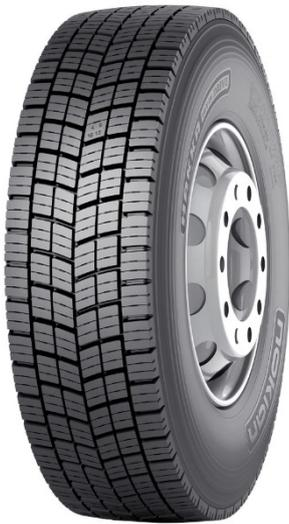
The Driving Safety Indicator (DSI), developed and patented by Nokian Tyres, also makes it easier to monitor the safety and wear of the tyre. It displays the remaining amount of tread surface on the tyre's main grooves in numbers.
